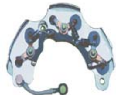
[Generator rectifier bridge] [40-8-9]
