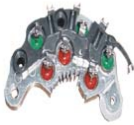
[Generator rectifier bridge] [cs130d]
