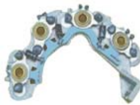
[Generator rectifier bridge] [50-8c]
