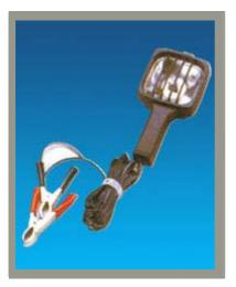
Product Line: Hand Held Spot Light Product Name: Work lamp KY-325 Specifications: Bulb Type :H3 12V55W Size:80x170x56(m/m) Packing:50 Pcs/CTN/3.6' Weight:16/17 Kgs Description: Housing:Hi Impact Grain Plastic Plug:Clincher
