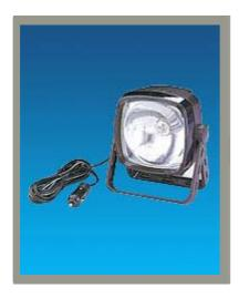
Product Line: Hand Held Spot Light Product Name: Work lamp KY-327 Specifications: Bulb Type :H3 12V55W Size:147x170x93(m/m) Packing:20 Pcs/CTN/2.3' Weight:13/14 Kgs Description: Housing:Hi Impact Grain Plastic Lens:Glass, Clear Plug:Cig. plug
